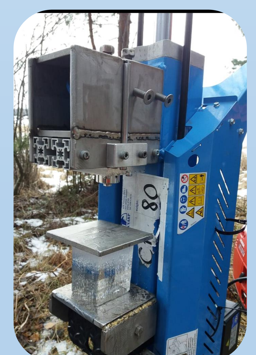
Fig. 11: Compressive strength test
