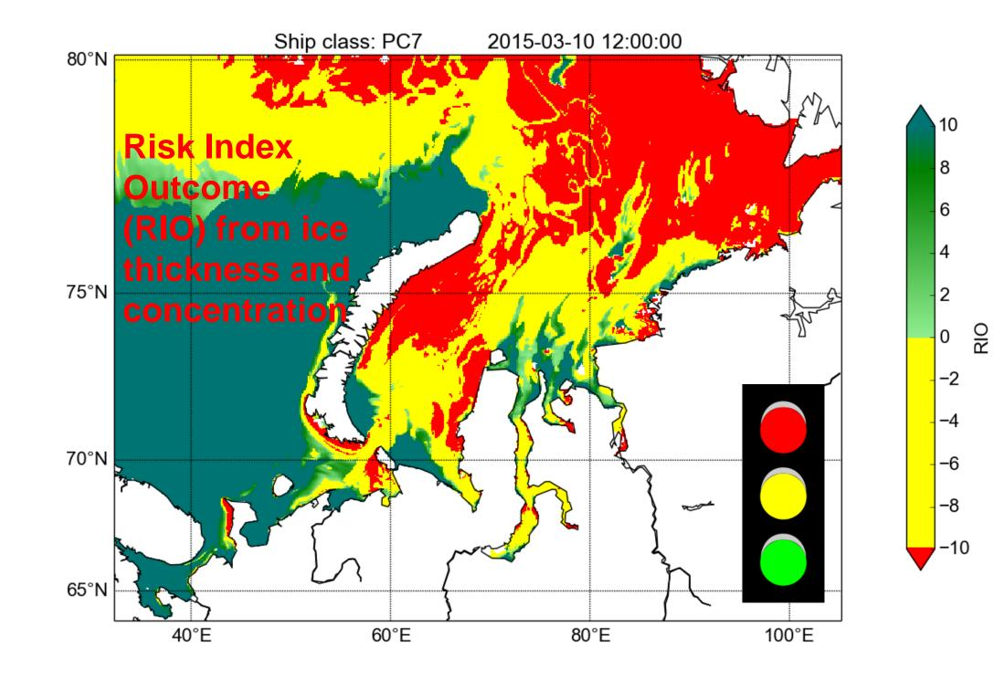
Fine resolution ice-ocean modelling of Kara-Barents sea and converting the results to forecast of ship specific navigability.
