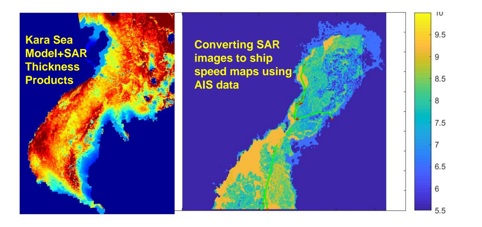
Combining thickness data from the ice model and satellite thickness data. Converting of SAR images to speed maps using observed ship response. Transfer of Baltic knowhow to the Arctic. Global AIS data: speeds and locations of all navigating vessels intergrated with the ice information
