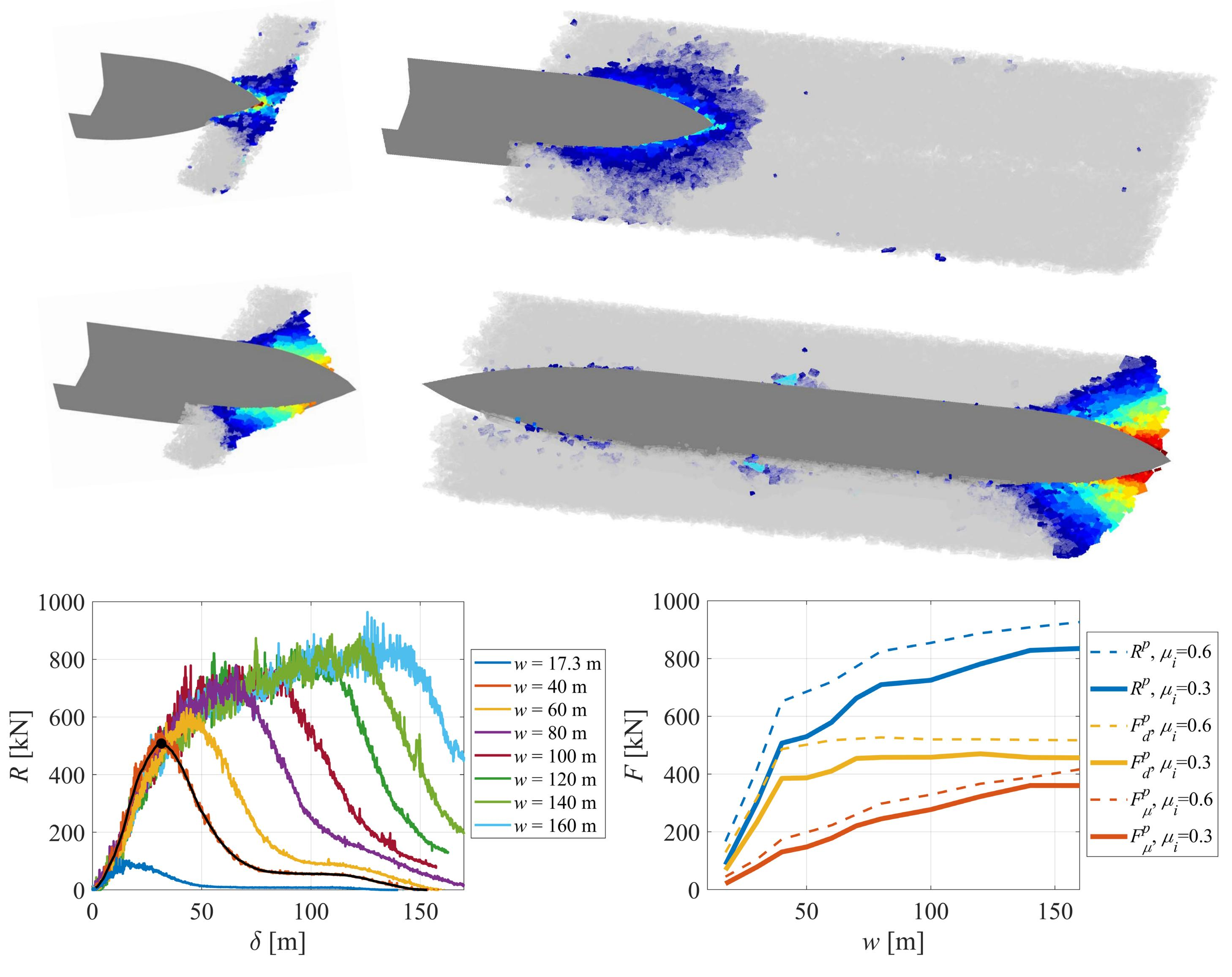
The ridge resistance-displacement  $(R-\delta)$  records from the simulations with different ridge widths w. The black line shows filtered data used to define the peak resistance  $R^p$  (black marker).
