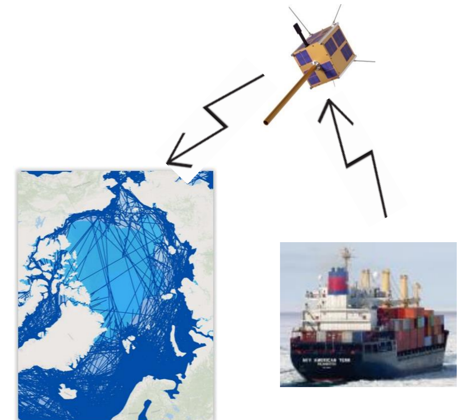
The locations and speeds of all ships navigating in the Arctic obtained from satellite AIS data
