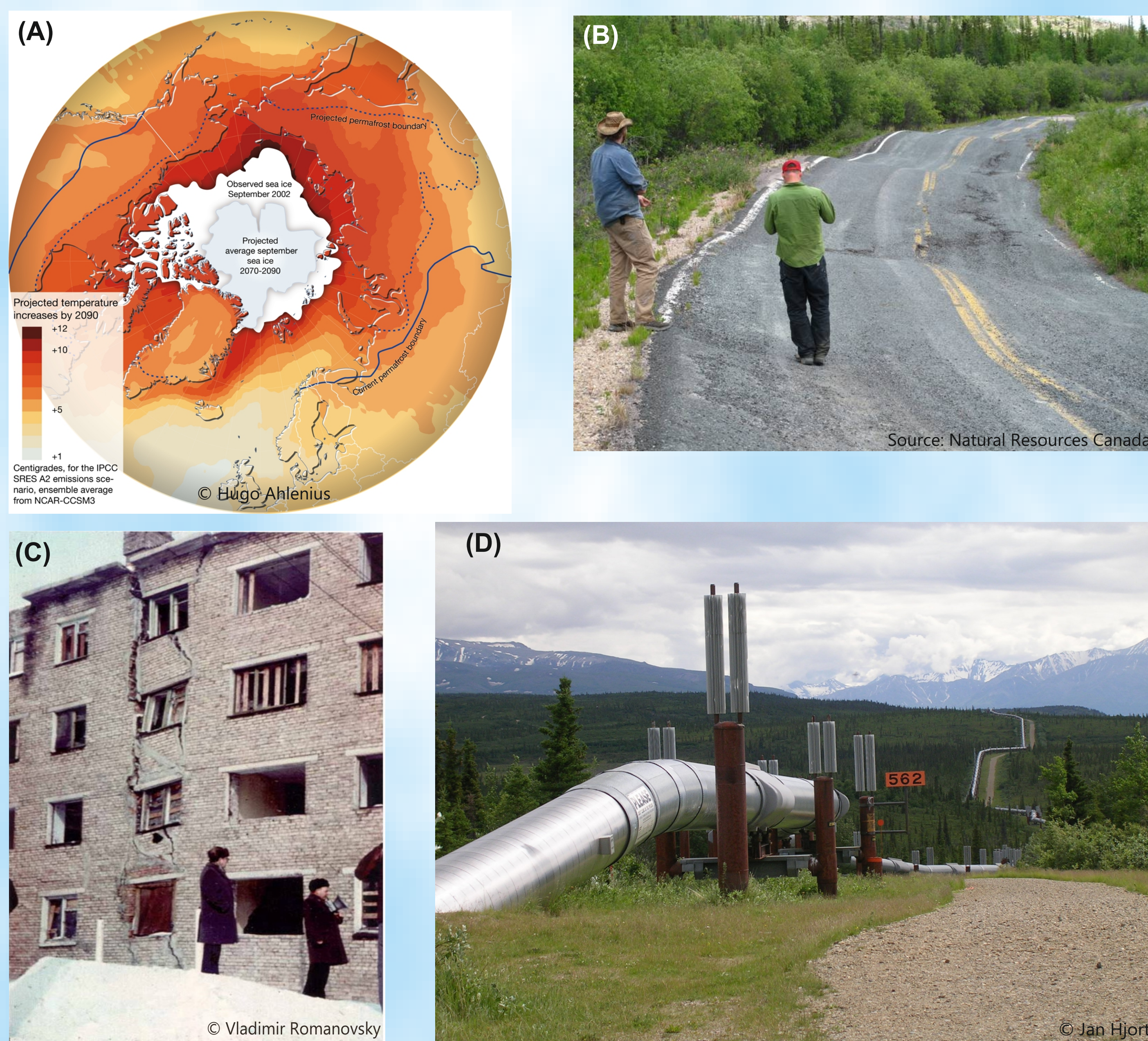
Figure 1. (A) Air temperature, permafrost and sea ice projections for 2090 (ACIA 2005). (B) Abandoned section of NWT highway 4 (east of Yellowknife) damaged by permafrost thaw. (C) A building buckled due to thawing permafrost. (D) The trans-Alaska oil pipeline.
