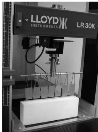
Fig. 2.7.1. Materials testing machine LR 30K for automatic dip coating.
