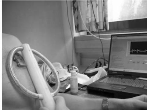
Figure 2.8.4. Testing of the operation of the first implant by recording surface ECG. The implant electrodes are pressed against skin.
