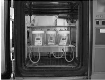
Fig. 2.7.4. Humidity and heating chamber for the permeability tests.
