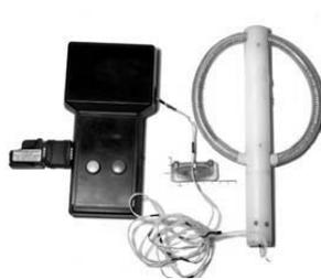
Fig. 2.8.2. Inductive reader unit for the first prototype. The coil antenna is constructed inside a plastic tube in a handle.
