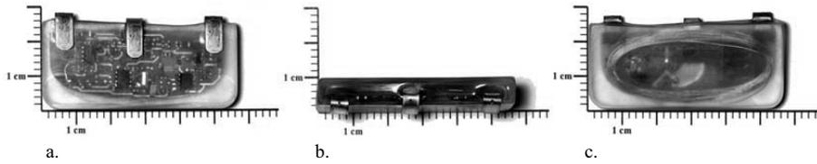
Fig. 2.8.1. Structure of the encapsulated first prototype device. a. Top view, b. side view, and c. back view of the device.
