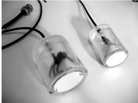
Fig. 2.5.13. Ultrasonic transducers used in the power transfer measurements.
