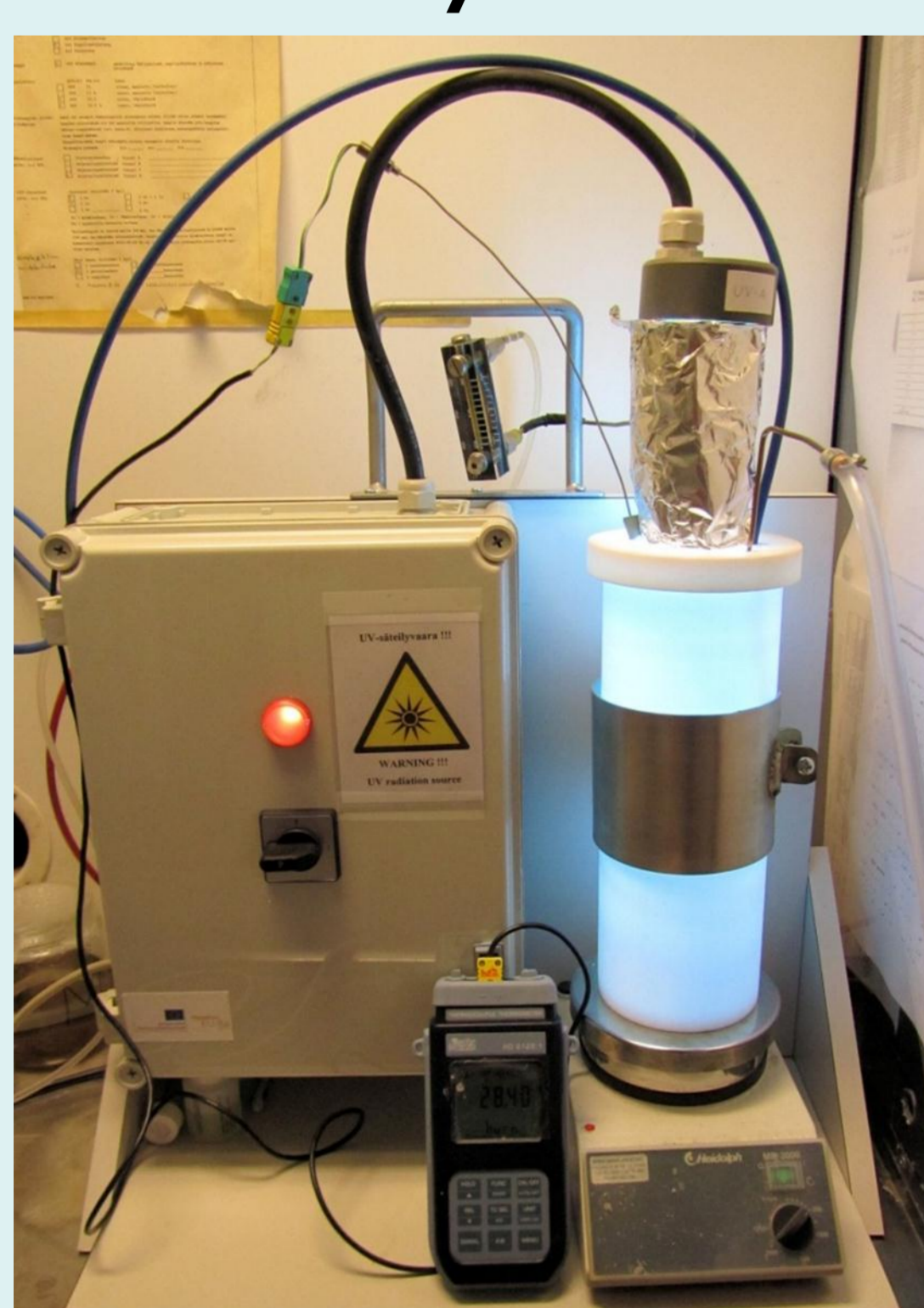
Figure 3. Equipment for the liquid phase photocatalysis studies.
