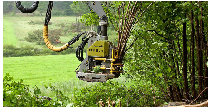
Multi-tree harvesting head. Photograph: Bracke Forest Ltd.
