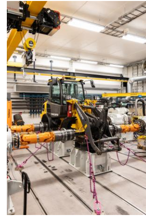
Picture 1. NUVE-LAB customized gears for single electric motor testing capability (left) and full electric mobile work machine testing set-up (right) in NUVE-LAB.
