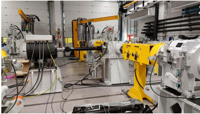
Picture 1. NUVE-LAB customized gears for single electric motor testing capability (left) and full electric mobile work machine testing set-up (right) in NUVE-LAB.
