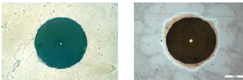
Figure 3. A nickel coated fibre (left) and a copper coated fibre (right) embedded using the nickel based brazing alloy MBF-35. The left result is excellent. The copper coated fibre is also well embedded, but the mixing of the coating and the brazing alloy is not as good as in the case of a nickel coated fibre.
