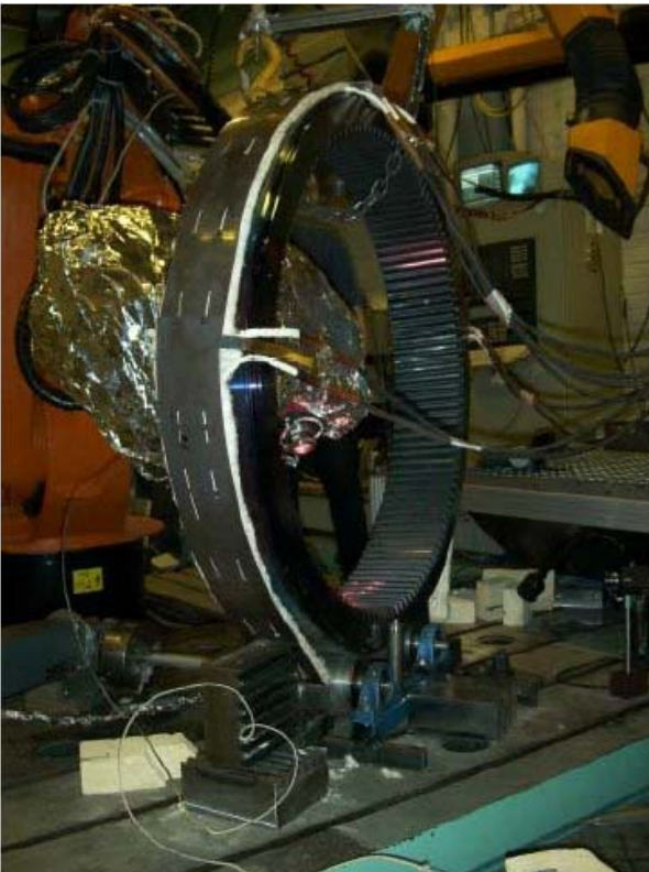
Figure 6. Ring gear hardening test setup.
