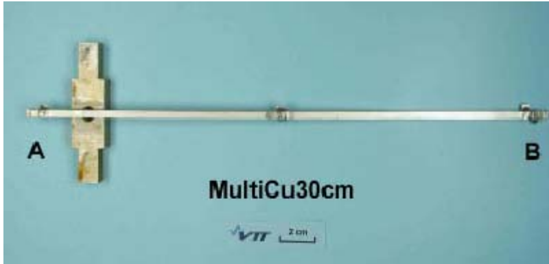
Figure 7. A specimen used for developing the brazing technique for long fibres, in this case a 30 cm long multimode copper coated fibre was embedded. The cross-section of the specimen is about 4×4 mm and the fibre is placed in the middle.
