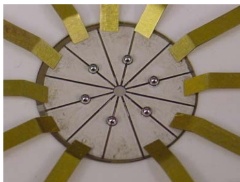
Figure 2. Prototype of the pre-stressed and curved piezoelectric stator ( \text{Ø}25 \text{ mm} ). 12 individual elements produce elliptical motion with the steel balls that are moving the rotor.
